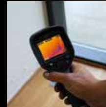
Find air infiltration problems
