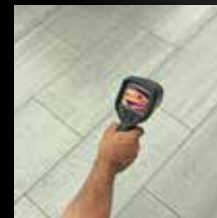
Check floorheating for leaks
